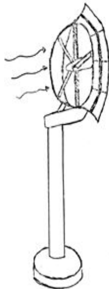
Figure 5: Downwind Turbine with Shroud to increase flow velocity through blades.
